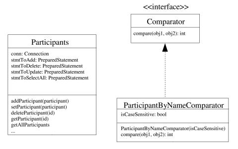
In a UML class diagram, the symbols are well defined. For example, the dotted arrow shown above means "implement an interface".
