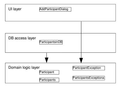
Now, the user interface layer only references the domain logic layer, but not the database access layer. Therefore, no matter the system uses a database, a text file or an XML file to store its data, this layer can be reused.
