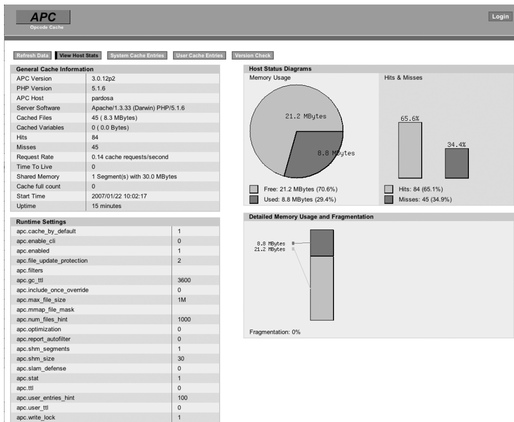
Figure 23-1. Alternative PHP Cache (APC) comes with an interface that displays memory allocation and the files currently within the cache.
