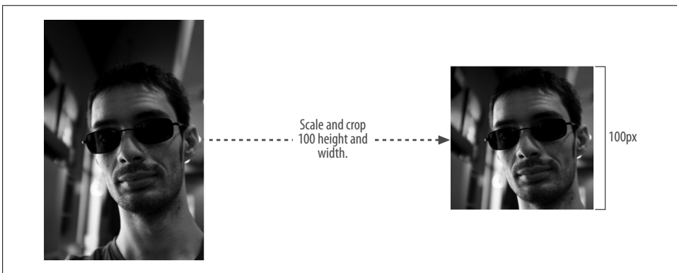
Figure 7-14. The scale and crop action trims off the larger side while maintaining the aspect ratio
